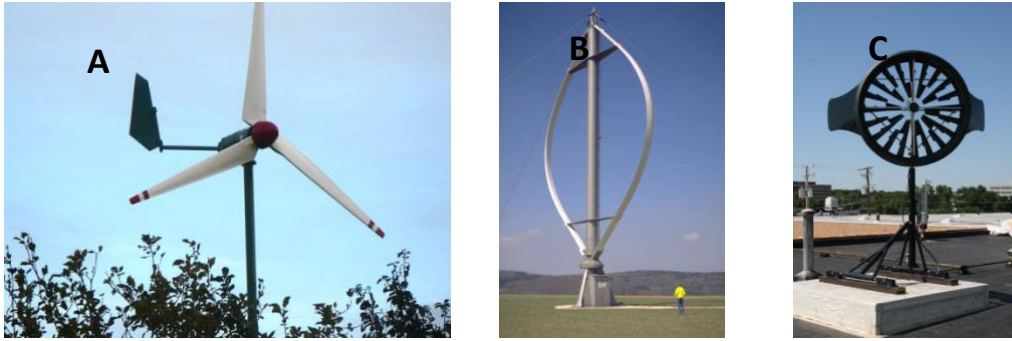
Figure 1137.01-A: Illustrative examples of the types of wind turbines, from left to right, (A) Horizontal Axis (HAWT), (B) Vertical Axis (VAWT), and (C) Blade Tip Power System (BTPS).
